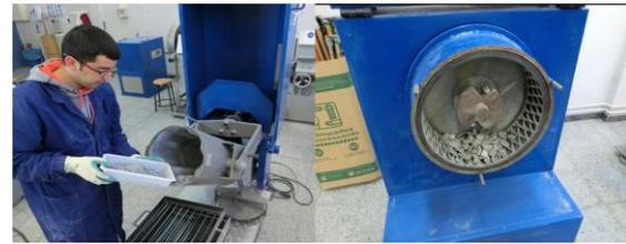
Preparing Bond rod mill test and Bond abrasion test.
