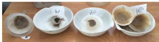
Photo: Filtered wet magnetic (MP), middle (ZP), nonmagnetic (UP) and rest (R) fraction taken after first separation trial.
